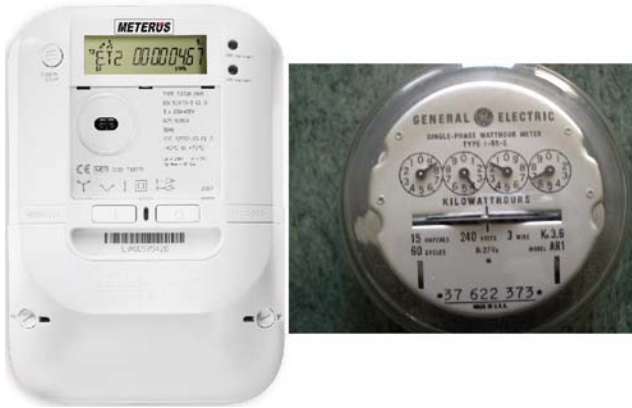
Figure 7 Smart Meter and Mechanical Meter 21+22
